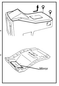
2 Holding up and remove the Screen Frame and then disconnect the connector of the Control Panel Board.
